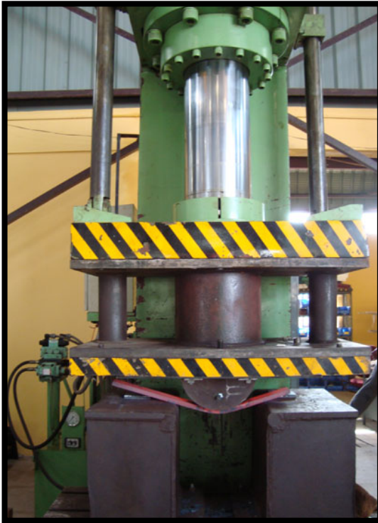
Clamps being hot formed in 150T press
