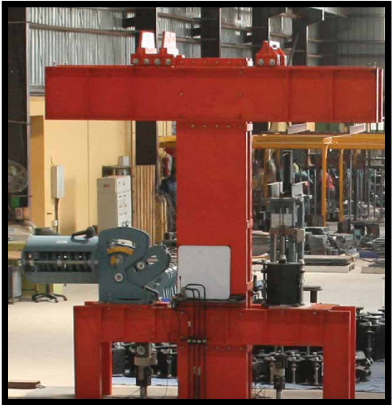
Constant effort support model HFMH & Variable effort support type D, under calibration test in our hydro mechanical test rig with load measurement by load cells and digital displays.
